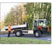
The hook devide can be operated with the Muli joystick inside the cab or outside with the RECON wireless remote control
